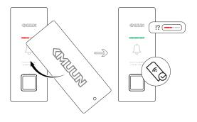
After setup any key, you may continue or exit. To add another key type, repeat the enrollment process. To exit, press the "Door Open Button" on the indoor unit.
