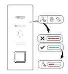
Fingerprint: Place your finger on the fingerprint sensor. Repeat the process until you see outdoor-all status LED show green, Setup succeeded
