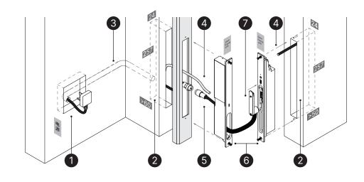
Once the power source location is set, an outlet 86 box is installed on the wall. The conduit between electric source and door leaf unit is then run to the door, making it ready for the final wiring.
